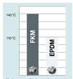
Maximum operating temperatures of the two different press-in branch connector types
