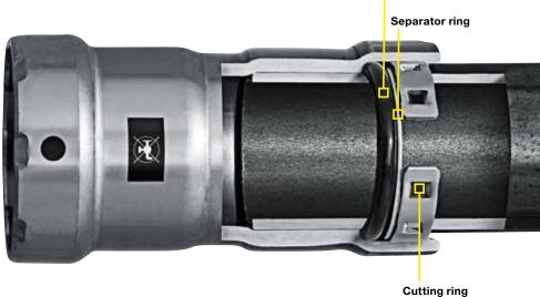
To prevent damage to the sealing element when the pipe is inserted, Megapress fittings up to 2 inches feature a protective separator ring. The cutting ring bites into the pipe during pressing and gives particular strength to the connection.
