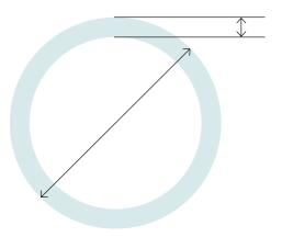
Pipe wall thicknesses and diameters according to DIN EN 10255, DIN EN 10220/10216-1 and DIN EN 10220/10217-1.
