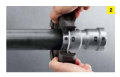
For pressing Megapress connectors from 11/4 inch upwards, only press rings with hinged adapter jaws are used. For smaller sizes between % and 1 inch, both press jaws and press rings with hinged adapter iaws are available.
