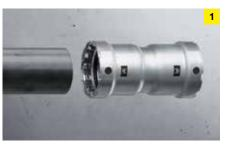
The steel pipe is cut to length and cleaned. Then the insertion depth is measured and marked, then the Megapress connector is put on the pipe up to the mark.
