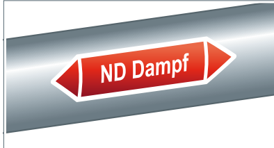
Fig. 152: Steam line with DIN 2403 marking
