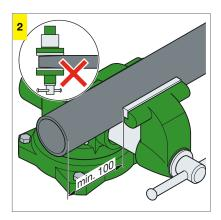
Proceed with caution when clamping the pipe – avoid deformation of the pipe end.
