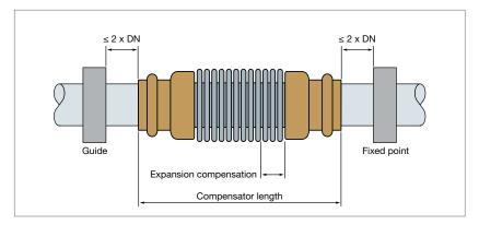
Fig. 55: Dimensions of axial compensators
