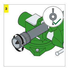
Use a deburrer to deburr the inside and outside of the pipe – up to DN40 use model 2292.2, DN50 use model 2292.4XLXL
