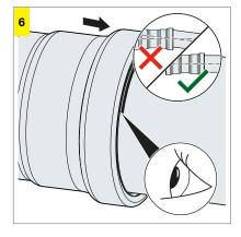
Push the press connector up to the marked insertion depth on the pipe.
