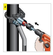
The hole is drilled by means of a commercially available drilling machine. The steel chips can be extracted by means of the vacuum cleaner nozzle. Afterwards, remove the drilling device again.
