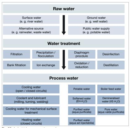
Fig. 88: Industrial process water supply
