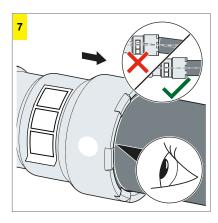
Push the press connector onto the pipe as far as it will go. Do not tilt the press connector. Check insertion depth.
