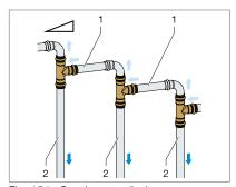
Fig. 154: Condensate discharge downwards
