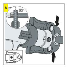
Place the Megapress press jaw (≤ DN25) around the press connector. Ensure it is properly seated. Carry out the pressing until the press jaw is completely closed.
