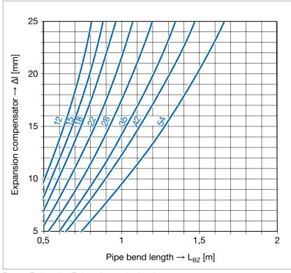
Fig. 79: Z-shaped or T-shaped expansion bend
