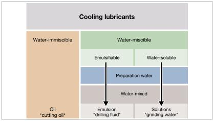
Fig. 166: Types of cooling lubricant (CL)
