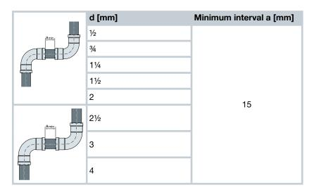
Tab. 13: Minimum space required between the pressings – press rings DN15–DN100
