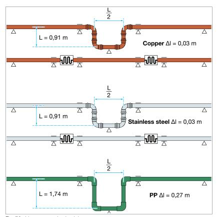
Fig. 76: Linear expansion in piping
