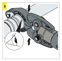
Attach the press machine and perform pressing.
