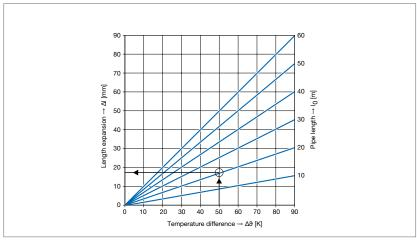
Fig. 34: Linear expansion of pipes made of copper and 1.4401 stainless steel
