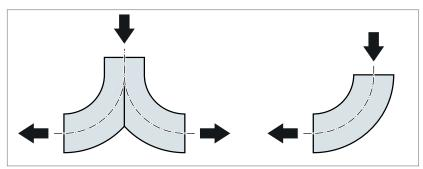
Fig. 132: Y-section and elbow
