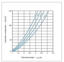
Fig. 45: Length determination for U-shaped expansion bend
