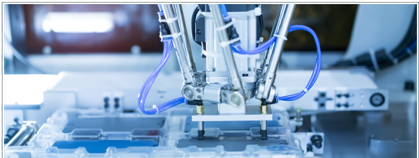
Fig. 121: "Pick and place" application using compressed air
