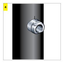
The steel pipe connection Rp ¾ for thermometers, temperature sensors, manometers, drains or line connections is completed.
