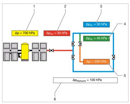
Fig. 130: Pressure losses from a compressed air system
