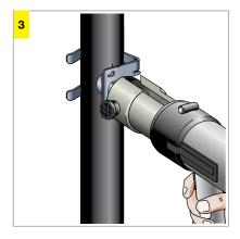
Press the press-in branch connector to the steel pipe by means of the press machine and the positioning aid. This is a fast and clean way of making the connection to the pipeline.
