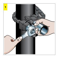
Fasten the special drilling device for guiding the drilling shaft to the steel pipe (1½-6 inches) using a ring or fork spanner.
