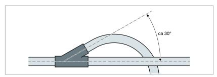
Fig. 133: Laying the connection line
