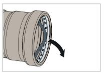
Fig. 15: Removal of the sealing element from XL press connectors – 64.0 – 108.0 mm
