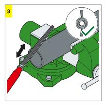
Properly deburr the inside and outside of the pipe.
