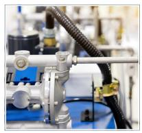
Fig. 120: Compressed air diaphragm pump
