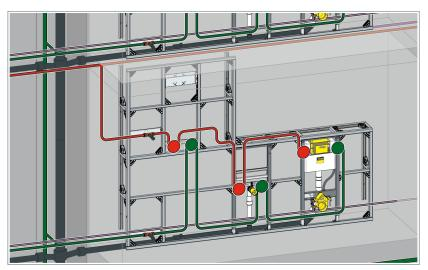
Fig. 83: Connection of a service unit to the potable water cold and potable water hot distribution, connection of the circulation outside the service unit.
