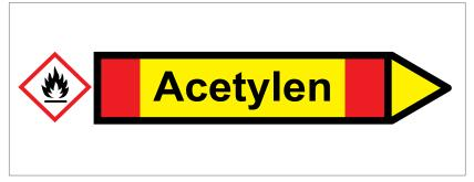
Fig. 139: Acetylene with hazard symbol
