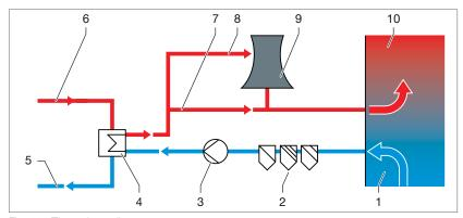
Fig. 93: Through-cooling
