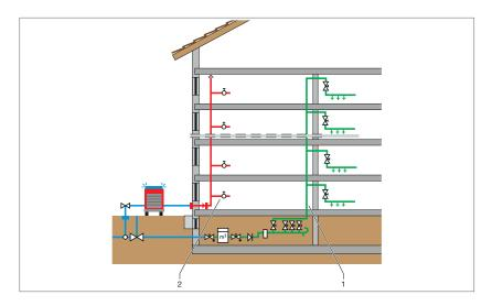
Fig. 110: Firefighting water system dry
