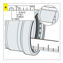
Mark the insertion depth on the pipe.
