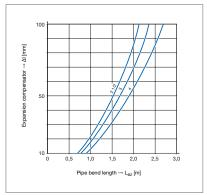
Fig. 53: U-shaped expansion bend for Megapress S XL 2½-4 inches
