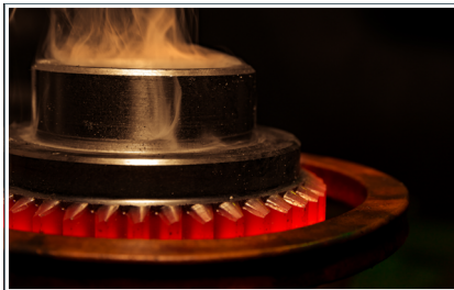
Fig. 136: Protective gas furnace for hardening gearwheels
