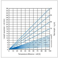
Fig. 46: Linear expansion steel pipes
