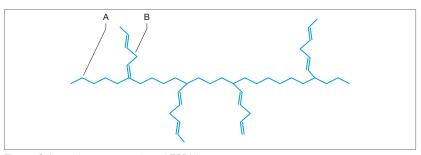
Fig. 3: Schematic representation of EPDM
