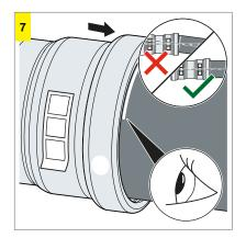
Push the press connector onto the pipe as far as it will go. Do not tilt the press connector. Check insertion depth.
