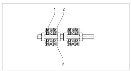
Fig. 7: Setup of the fixture for determining the compression set according to ISO 815
