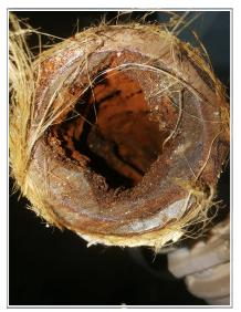
Fig. 74: Galvanised steel pipe with clearly visible corrosion
