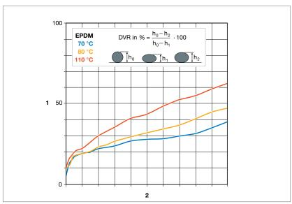
Fig. 9: Compression set for a selected EPDM at different temperatures
