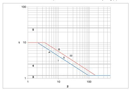
Fig. 145: Operating ranges according to the hazard in case of acetylene decomposition (Source: EIGA IGC Document 123/13/D)
