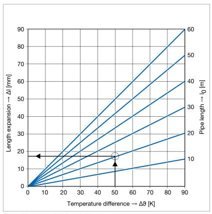
Fig. 78: Linear expansion of metal piping
