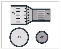
Fig. 126: Flow behaviour in case of changes to the cross section
