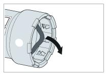
Fig. 22: Removal of the sealing element from press connectors – up to 2 inches
