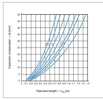
Fig. 52: U-shaped expansion bend for Megapress/Megapress S %-2 inches
