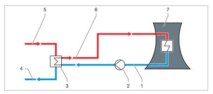
Fig. 95: Closed cooling circuit with circulation cooling
