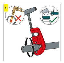
Cut the steel pipe properly and at a right angle using a pipe cutter, angle grinder or finetoothed hacksaw. Do not use a flame cutter.
