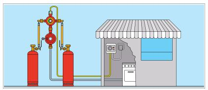
Fig. 146: Liquid gas cylinders
