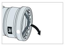
Fig. 25: Removal of the sealing element from press connectors – from 2½ inches
