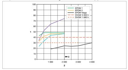
Fig. 10: Compression set for various EPDM types at the same temperature during the test procedure according to DIN EN 681-1
