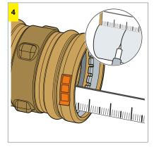
Mark the insertion depth on the pipe.
