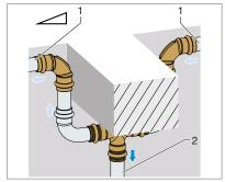
Fig. 157: Bypass around an obstacle
