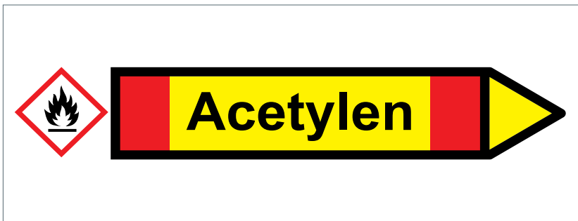
Fig. 139: Acetylene with hazard symbol
