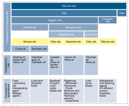
Fig. 158: Classification of oils and typical applications
