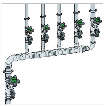
Fig. 80: Hygienically optimised manifold installation
