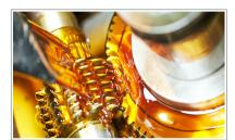
Fig. 164: Application of a cooling lubricant
