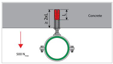
Fig. 113: Steel dowel without fire protection proof of suitability
