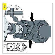
Place the Megapress press ring around the press connector. Ensure that it is properly fitted. Carry out the pressing using the hinged adapter jaw until the press ring is completely closed.
