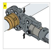
Attach the press machine and perform pressing.
