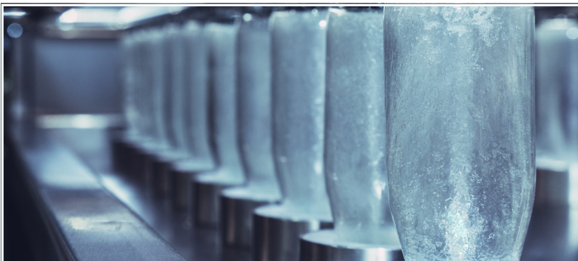
Fig. 102: Water heated by process heat for cleaning bottles
