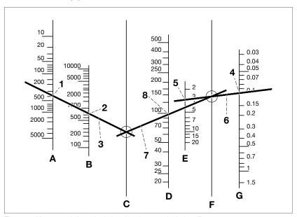
Fig. 131: Nomograph for calculating the clear nominal pipe diameter
