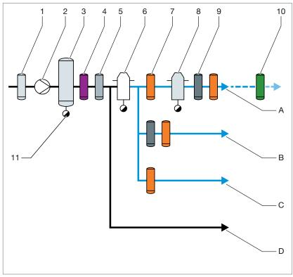
Fig. 127: Principle of a compressed air system
