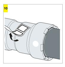
Remove the control label to mark the connection as "pressed".
