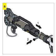
Place the Press Booster in the press machine and lock in place using the retaining bolt.
