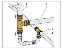
Fig. 156: Condensate loop – separation of steam and condensate
