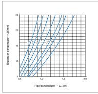
Fig. 50: Z-shaped and T-shaped expansion bends for Megapress/ Megapress S %-2 inches
