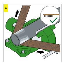
With the help of a wire brush, sanding paper or an angle grinder with a fan washer, remove loose dirt and rust particles from the pressing area.
