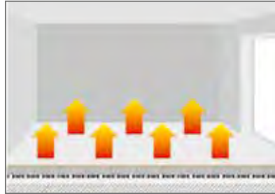
Fig. 21: Convection of underfloor heating
